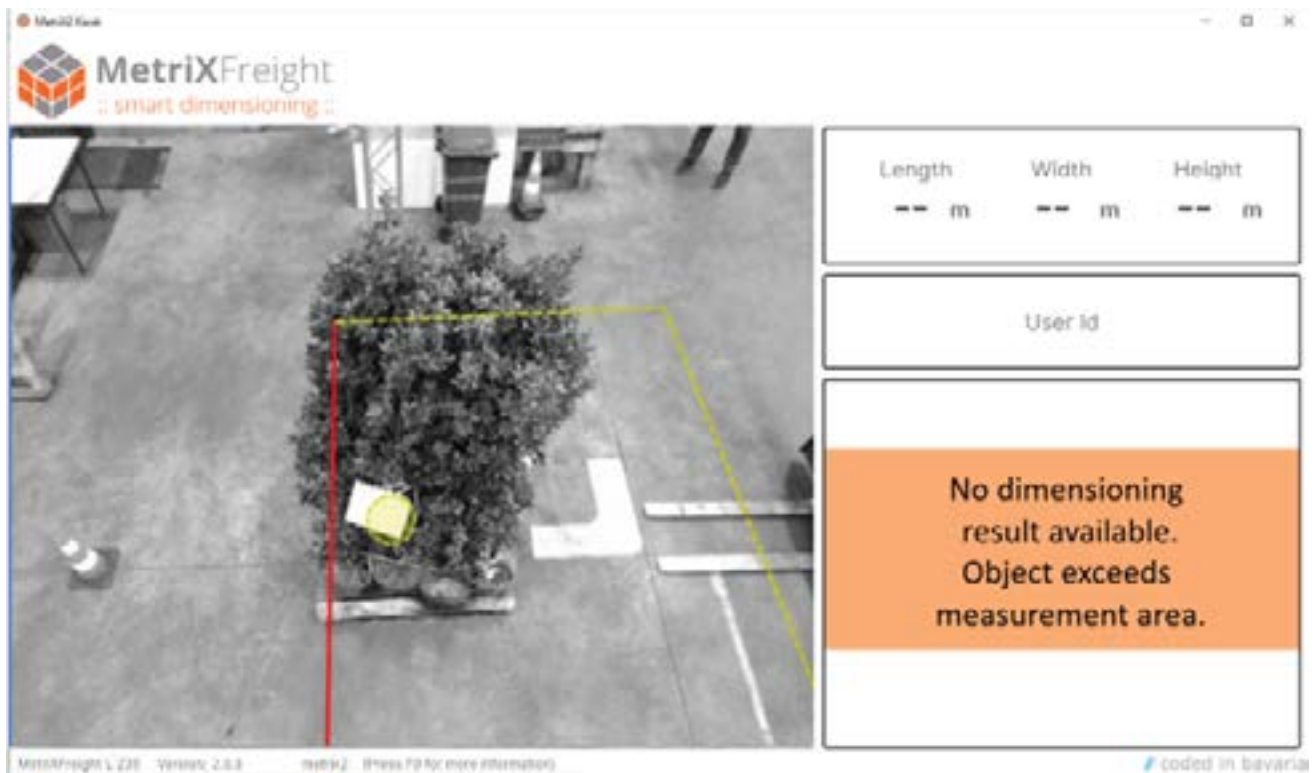
Figure 3: An object is misplaced and exceeds the measurement area on one side. An error message is shown, and the violated side is colored in red.
