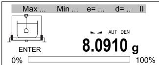
Hang plunger in liquid – measurement in liquid – and press *ENTER*.
