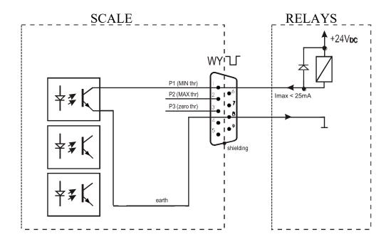
Relays output is the open collector transoptor output with load capacity 25mA / 24V. Transmitter inputs must be protected with diodes, e.g. 1N4148.
