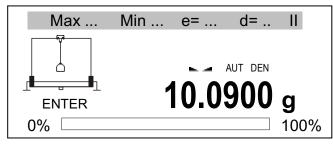
Hang plunger (without diving it in liquid) – measurement in air – and press *ENTER*.
