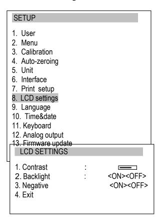
LCD settings enable to set contrast and backlight.
