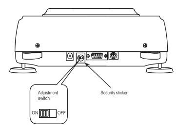
In balances comply with verification requirements performing calibration requires changing adjustment switch position, which is placed behind protecting mark (sticker) of a notified body. An access to the switch is possible only after removing the mark.
