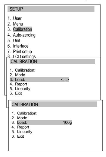
Load option enables inscribing standard of mass value, which will be used to calibrate (it is suggested to use standard of mass value close to balance's max).
