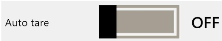
Tare on stability: When this function is activated, the equipment must show a stable reading when a tare is set. With the "OFF" option, the equipment tares under any stability condition.
