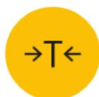
Pressing this key activates the tare function: The scale stores the weight currently on the load receptor and subtracts it from the total weight until the tare function is deactivated or cancelled. The tare function is active only when the weight is stable. If the stability indicator is off, pressing this key has no effect.
