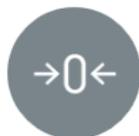
also deactivates the tare if it is activated. The zero setting of the scale is limited to the value indicated in the "Initial zero setting range" menu, which is the percentage over its maximum capacity. If this range is exceeded, the error message "Err0" is displayed.
