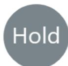
Pressing this key activates the "HOLD" mode. The display remains frozen at the current reading to indicate that the function has been activated, and the key remains in light grey. To deactivate it, press it again. When this mode is activated, the display always shows the weight of the last load on the pan. This means that even if you remove the load from the pan, the display will still show the last weight displayed.
