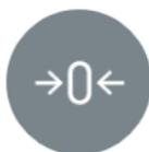
When this key is pressed, it is reset to zero. The scale is considered to be "at zero" when the weight on the load receptor is less than  $\frac{1}{4}$  of the division or resolution. While the scale is being zeroed, the display shows
