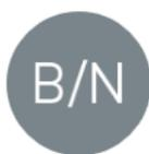
When the tare function is activated, the gross or net weight is displayed alternately. The display indicator
