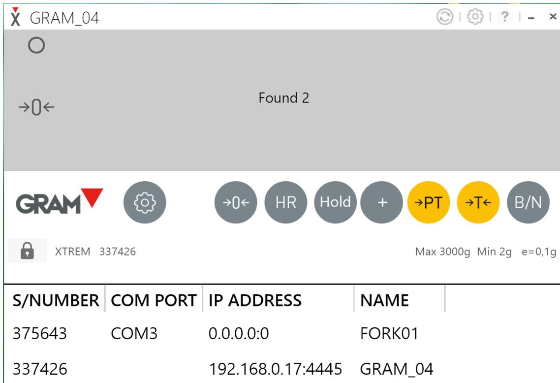
Automatic zeroing at start-up requires the balance to remain stable for at least 5 seconds.
