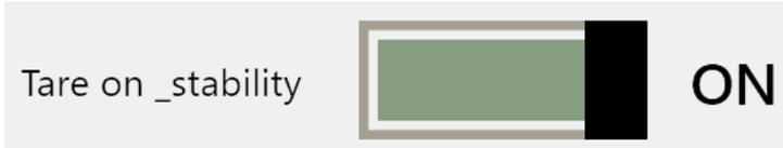
Preset tare mode: With the "ON" selection, the instrument remains tared after the load receptor is emptied. When the scale is emptied, the display shows the tare value with a negative sign. If you select "OFF", the tare is automatically switched off when the weighing platform is emptied.
