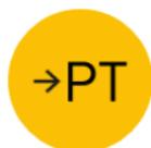
Pressing this key opens a dialog for entering a manual tare value using the numeric keypad. This value is subtracted from the weight value of the platform. To cancel it, press the key
