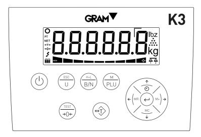
**Turn on/off the equipment.** When pressed, it turns on the indicator. When the indicator is on, pressing and holding it for two seconds turns it off.
