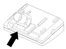
Slide the bracket between the two guides on the indicator box and push until the safety stop engages.
