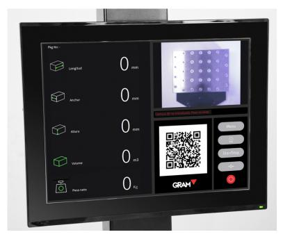
The upper right part shows the platform, where the package or box to be checked should be placed.
