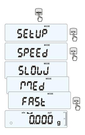
Option enables to change weighing speed, that enables better performance thanks to adaptation to environment conditions.
