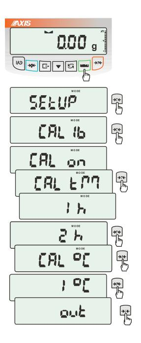
Press *MENU* key to display function menu and choose *CALIb* function by pressing  $\rightarrow T \leftarrow$  key when it is displayed. The following options will appear:
