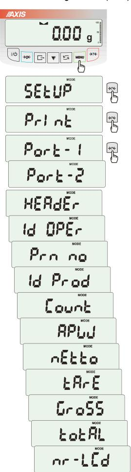
Function is used for printing additional information stored in scale memory, weighed product identification data and scale operator id. That information is inscribed using scale keys or scanner.
