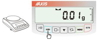
If the scale is not loaded and  $\rightarrow 0 \leftarrow$  indicator doesn't indicate, press  $\rightarrow 0 \leftarrow$  key.
