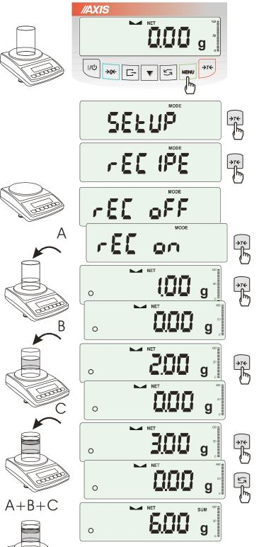
The function allows for separate weighing of several ingredients in one container with the possibility of reading current sum of all weighed ingredients.
