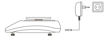
Plug feeder into ~230V power supply socket. When the pan is empty plug feeder output connector into 12V socket at back of the scale. Autotests and internal calibration will be performed.
