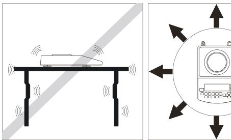
Location for the scale should be chosen with care in order to limit influence of the factors that can interrupt working scale. This location has to maintain proper temperature for working scale and necessary space for its operating. The scale should stay on stable table made of material that does not influence magnetically on the scale.
