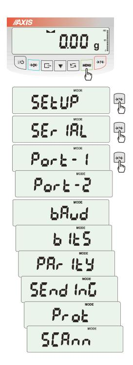
The function allows setting independently communication parameters of both of serial ports *Port-1* and *Port-2* (executed in RS232C, RS485, USB or LAN standard):
