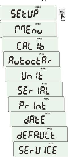
SEtUP contains all options used for setting scale work mode:
