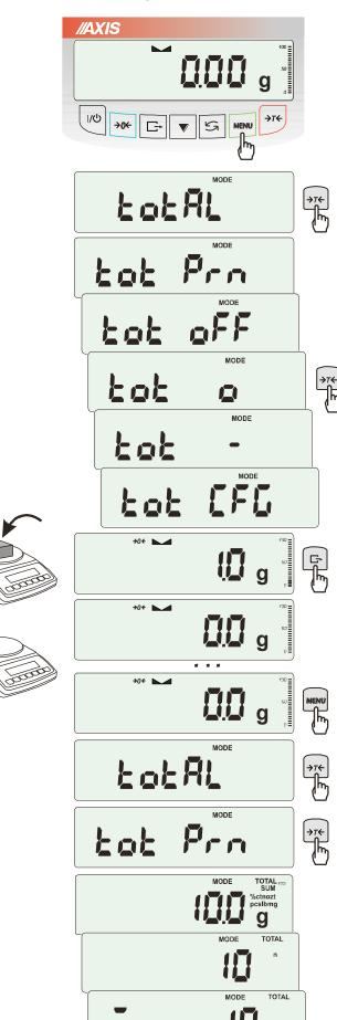
The function allows calculating total weight for series of measurements, which can be greater than scale capacity. It allows calculating total weight as well as average value.
