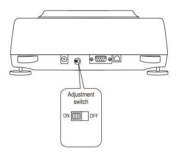
In balances comply with verification requirements performing calibration requires changing adjustment switch position, which is placed behind protecting mark (sticker) of a notified body. An access to the switch is possible only after removing the mark.
