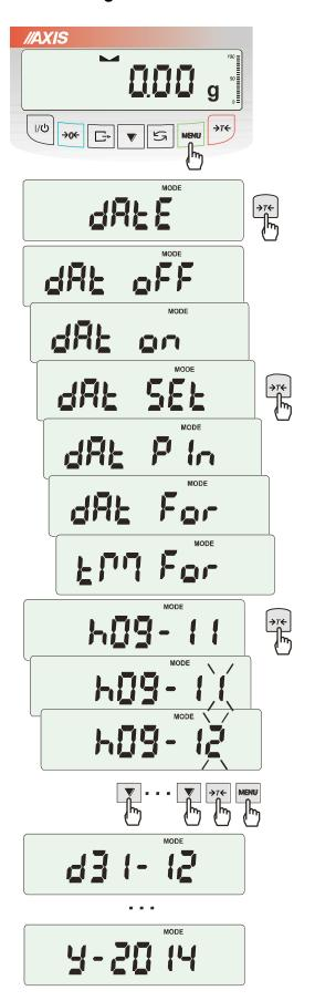
The function allows setting current date and time of scale internal clock and mode of its use.
