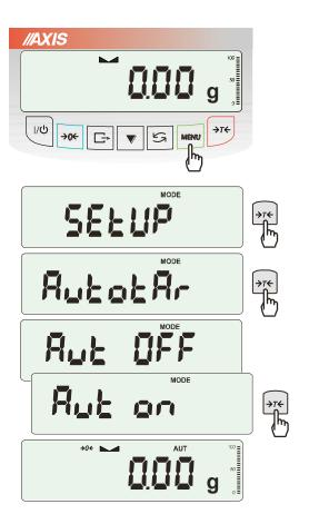
When the function is activated, the scale automatically ensures stable zero indication if the pan is empty or if zero indication was acquired by pressing  $\rightarrow T \leftarrow$  key.
