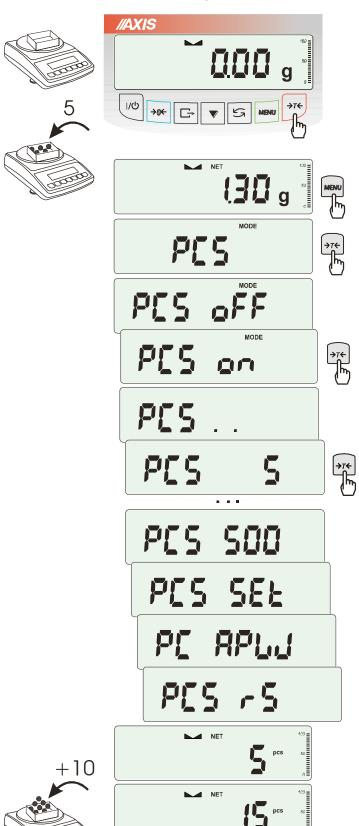
This function enables to count identical pieces, e.g. turnbuckles or buttons.
