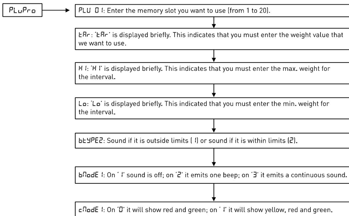
Weight limit function helps to indicate if a weight is within a particular range, transmitting a visual signal through the colours on the display and the bottom bars of the display with the option of also sending out a sound signal through the indicator.
