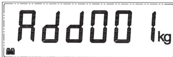
To add the weight of another object, the previous one must be removed. Make sure the display has returned to zero and the stability symbol is on. Only then can the operation be repeated.
