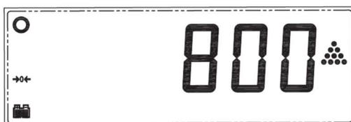
Place the pieces you want to count on the weighing platform (they should have the same individual weight as the previous sampling). You can place the pieces inside a container if its tare is already set up (check the Using the Tare section).
