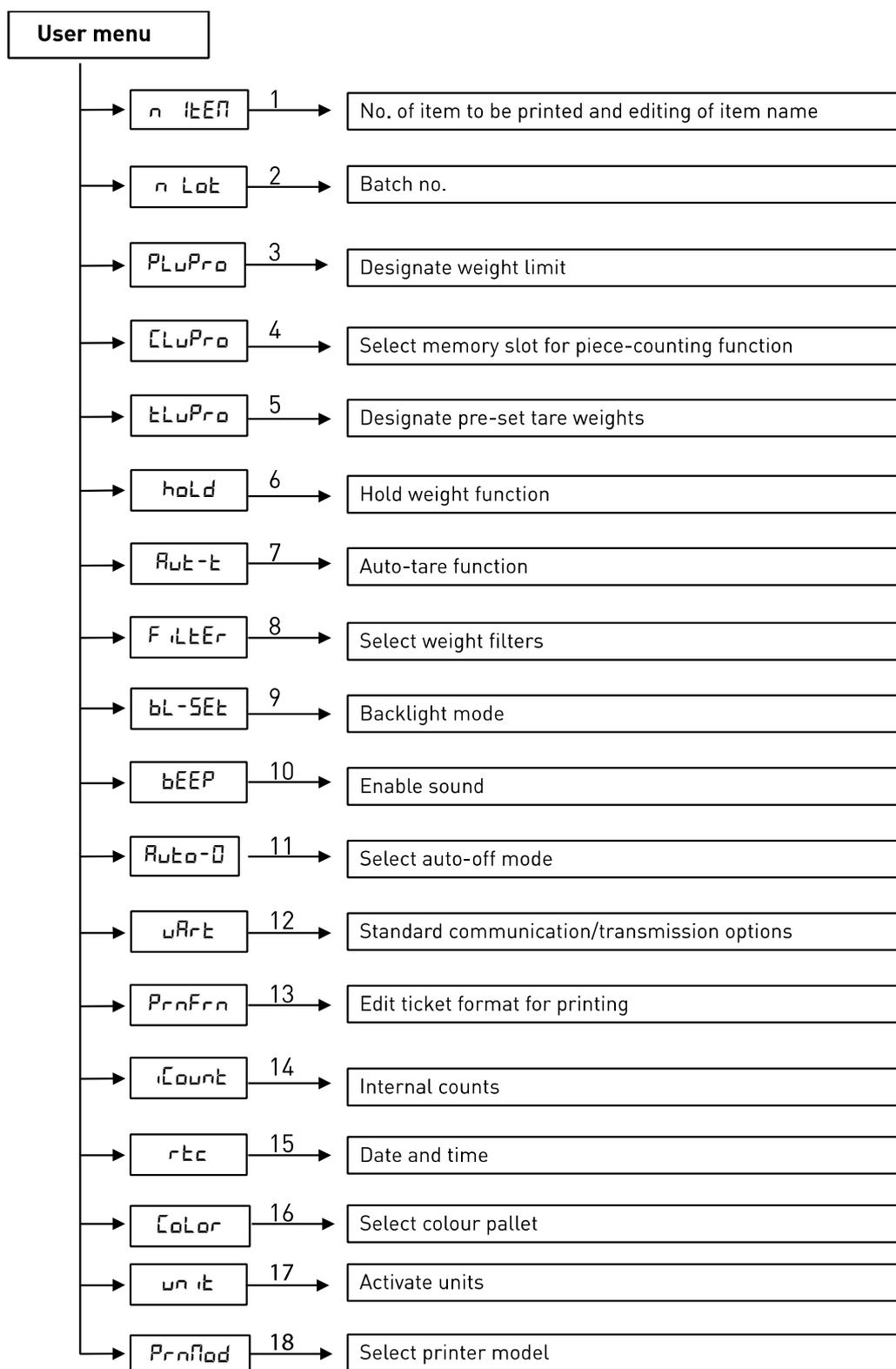
To access the functions set up menu, press the
