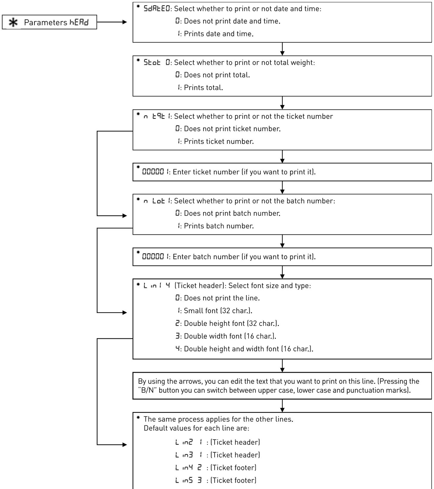
The printer data output can be set up with 5 different printing formats, according to the following versions:
