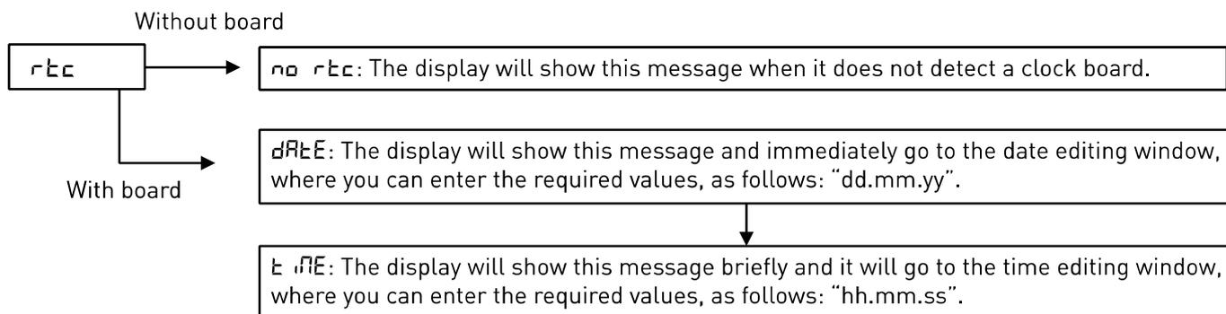
This function allows you to set the date and time if the device has our clock board.
